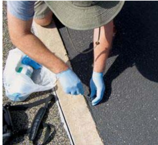
A city scientist collects a sample of paving sealant from a parking lot in Southwest Travis County. Tests showed it was not coal tar, as indicated by the gray color. Coal tar lots are blacker in color.
